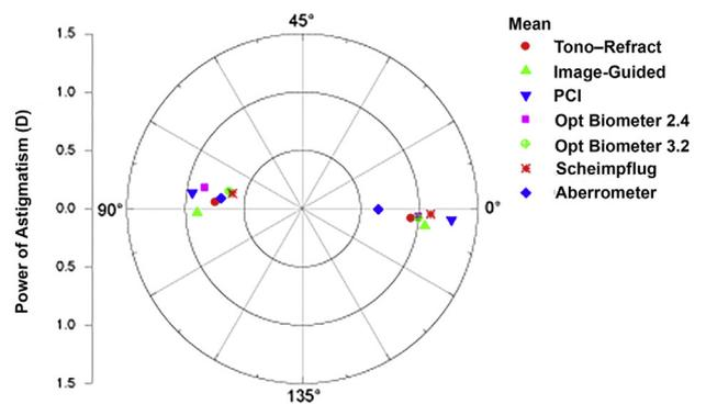
**Figure 3.** Double-angle plots for all 6 devices showing the mean astigmatism results of both groups (WTR and ATR on the right and left side, respectively). Polar plot with power of astigmatism (radius) versus axis (angle) (Opt = optical; PCI = partial coherence interferometry biometer; Tono-Refract = tonometer–refractometer).
